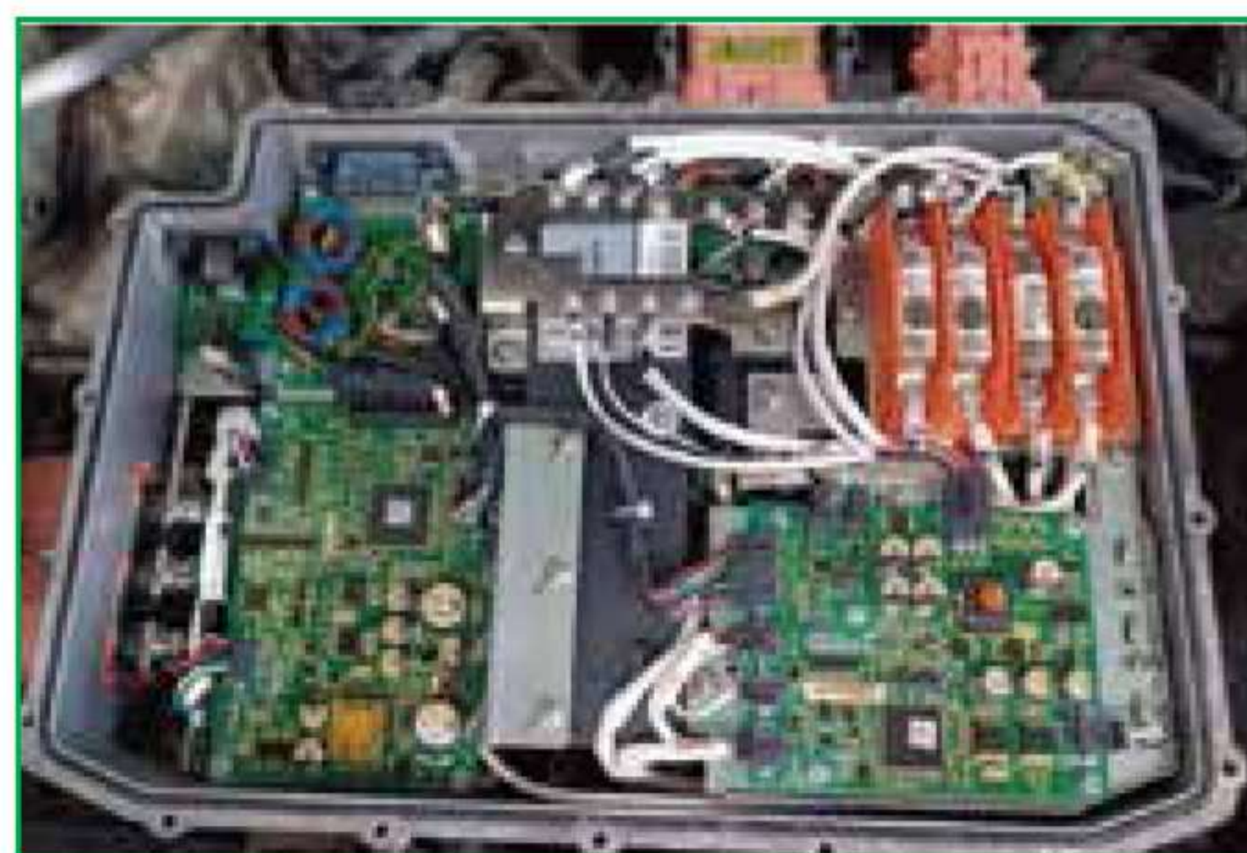
Precharge resistor, reverse diode burned out
